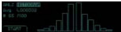
View results in Histogram mode to reveal stability or noise problems in analog circuits
